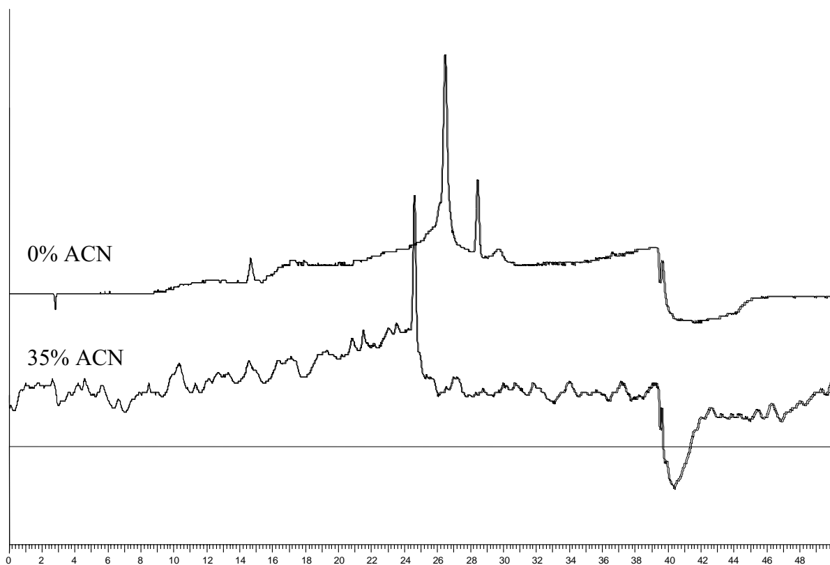
Fig. 5. Comparison of baseline noise between 0% acetonitrile and 35% acetonitrile in the mobile phase. The y-axis is response in mV, and x-axis is retention time in minutes.
